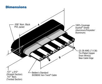
NOTE: the transition area is included in the twisted section to assure a full 2 Inches of flat termination area.
