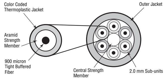
**Breakout Style Cable**Tight Buffer — Indoor Riser, Plenum & LSZH Rated (*continued*)
