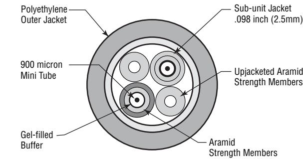
**Micro Loose Tube Breakout Style Cable**Loose Tube – Outdoor, Indoor/Outdoor OFN & Indoor/Outdoor Riser Rated (*continued*)
